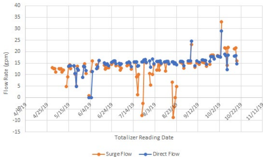
Figure 2-1 Daily Linear Hydraulic Loading Rates
