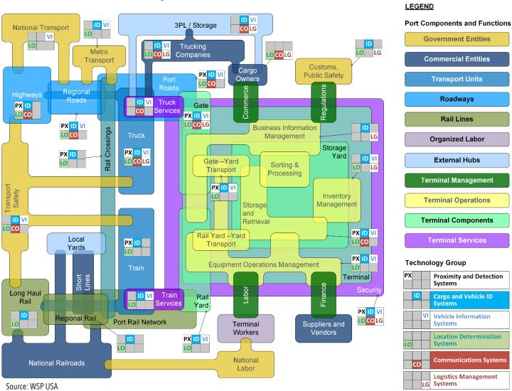
Exhibit 4 presents the logical relationship between the major elements of a port, its landside connectivity, its operating components, and the entities with which it interfaces. Shape overlaps reflect interactions between elements. Wherever ITS technologies might have a role or influence, an icon indicates those technology classes that are likely to be deployed in support of more efficient and safer operations.
