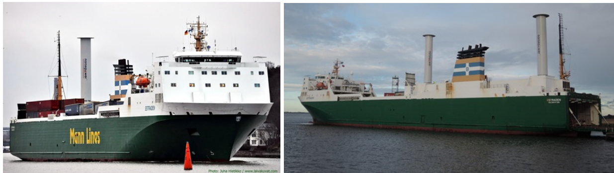
Figure 69 Norsepower Rotor Sail installation on the M/V Estraden . The left image shows the first installation from 2014, and the right image shows the second installation from 2015. Source: [Ref. 73].
