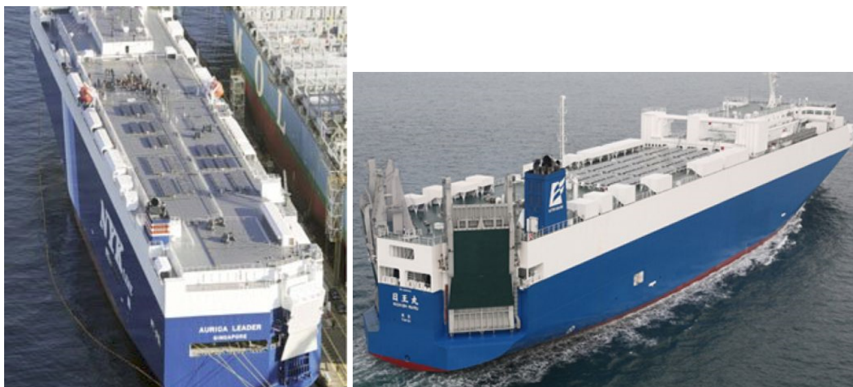
Figure 38 NYK (left) and Nissan (right) have both retrofitted large car carriers with solar panels
