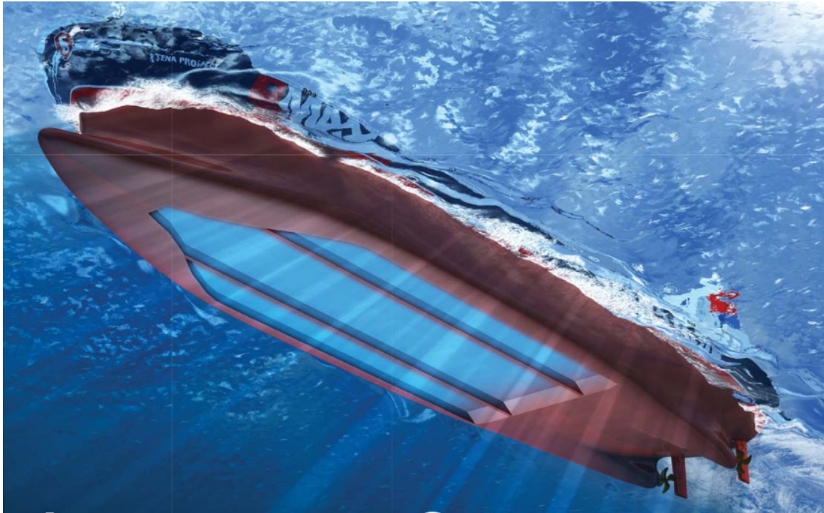
Figure 66 The Stena AirMAX developed by Stena Bulk is an air-filled cavity under the vessel. Source: [Ref. 15].
