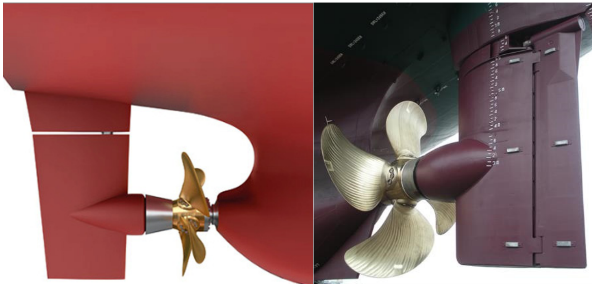
Figure 15 Rolls Royce Promas rudder (left) and Wärtsilä Energopac rudder (right) integrates a Costa bulb, rudder cap, and twisted rudder into a single device
