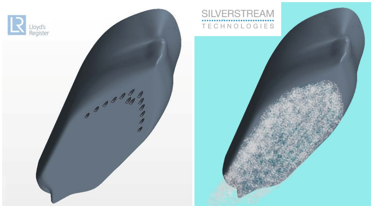
Figure 64 The Silverstream system injects micro-bubbles from air cavities installed near the bow of the ship (Source: Silverstream Technologies Ltd.)
