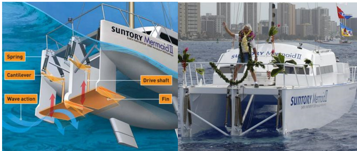
Figure 31 In 2008, the wave-powered Suntory Mermaid II sailed from Hawaii to Japan. Source: [Ref. 20]
