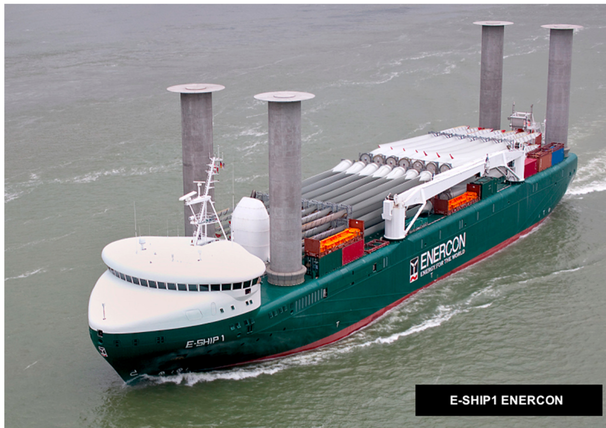
Figure 21 Enercon E-ship1 utilizing four Flettner Rotors. Source: [Ref. 54]
