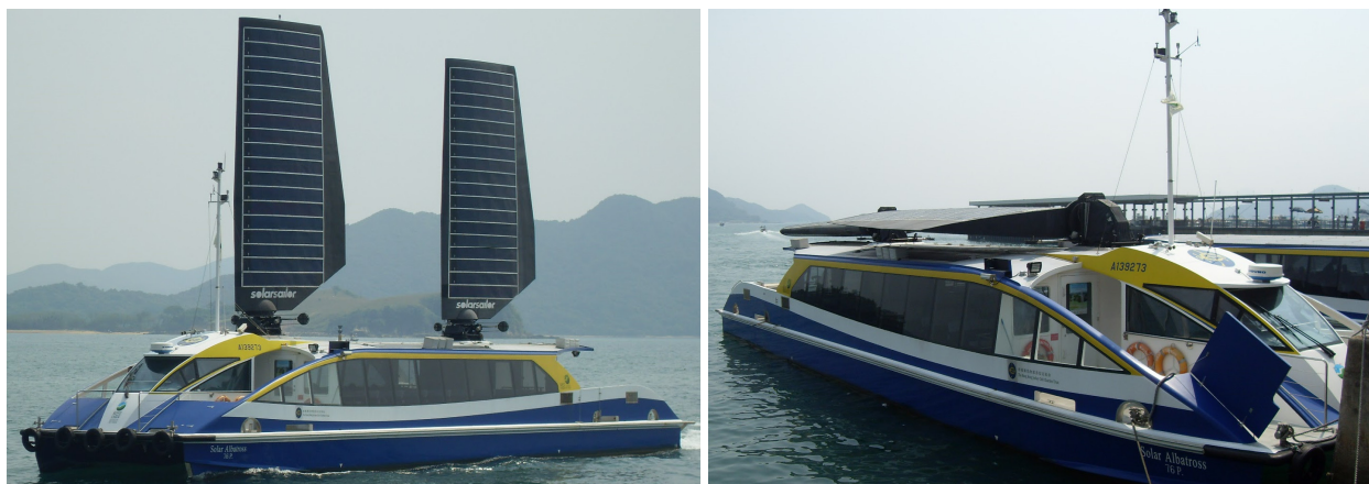
Figure 37 The Solar Albatross uses two retractable wingsails and solar arrays for propulsion. (Source: Ocious®)
