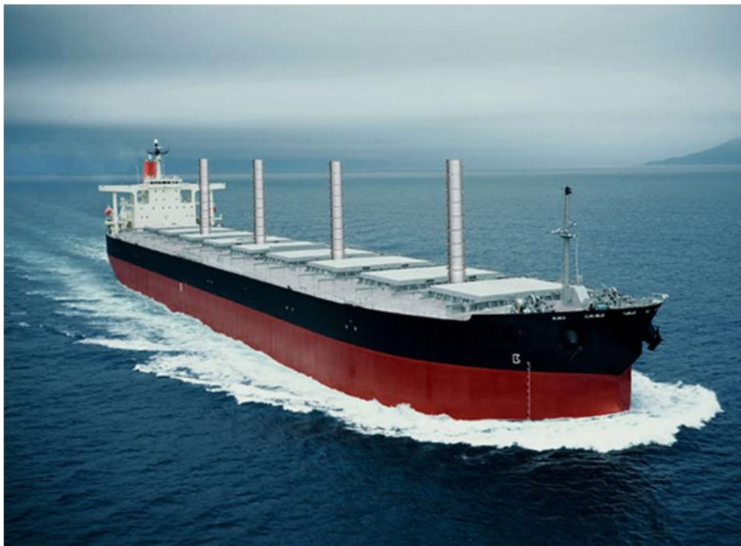
Figure 72 Magnus VOST™ rotors depicted on a large bulk carrier. (Source: Magnuss Ltd.)
