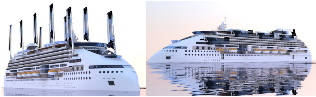
Figure 39 The Ecoship is a hybrid cruise ship concept utilizing unprecedented levels of solar, wind, and biofuel for vessel operations. Source: [Ref. 28].
