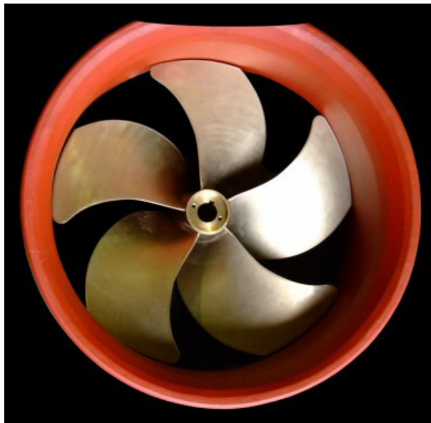
Figure 7 A ducted propellers (Kort Nozzle) can increase propeller efficiency at lower speeds. (Source: Maritime Professional).
