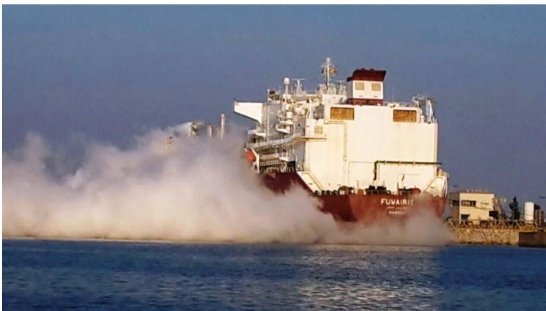
Figure 4. White cloud formed during the release of LNG.
