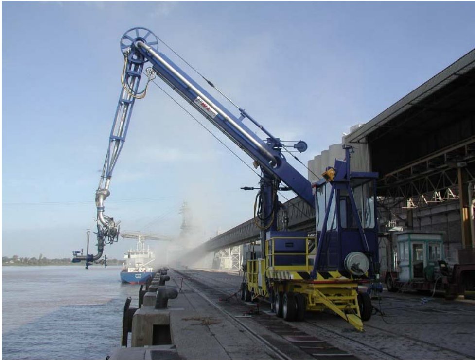
Figure 19 Mobile marine loading arm (Wiese Europe)
