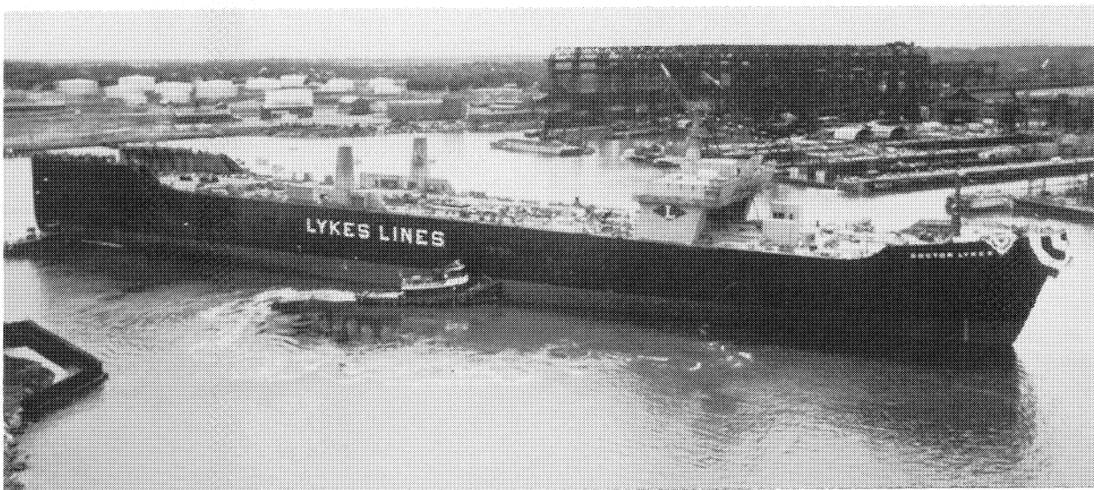
The largest dry cargo ship in the world is the SS DOCTOR LYKES. The 875-foot long carrier and two sister ships are being built for Lykes Bros. Steamship Co., Inc., by the Quincy Shipbuilding Division of General Dynamics.
