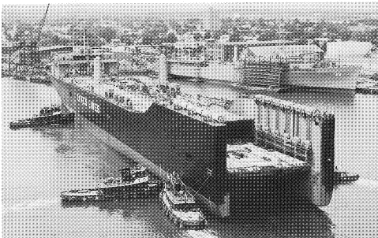
The stern view of the DOCTOR LYKES during its launching shows the elevator to which barges are floated and then raised to the section of the ship in which they will be carried. This type of vessel can lower the elevator offshore and discharge floatable barges thus decreasing costly port time of the vessel.
