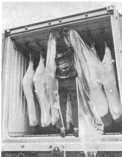
Innovative container developments, such as this temperature-controlled hanging-meat container, improve the competitiveness of American container operators.
