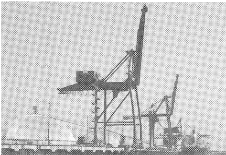
Two cranes are poised for action as third works ship in Port of Tacoma, Wash. Forty-ton container crane at left is new. Domes behind cranes hold imported alumina awaiting transshipment to Kaiser Aluminum plants in Tacoma and Spokane.
