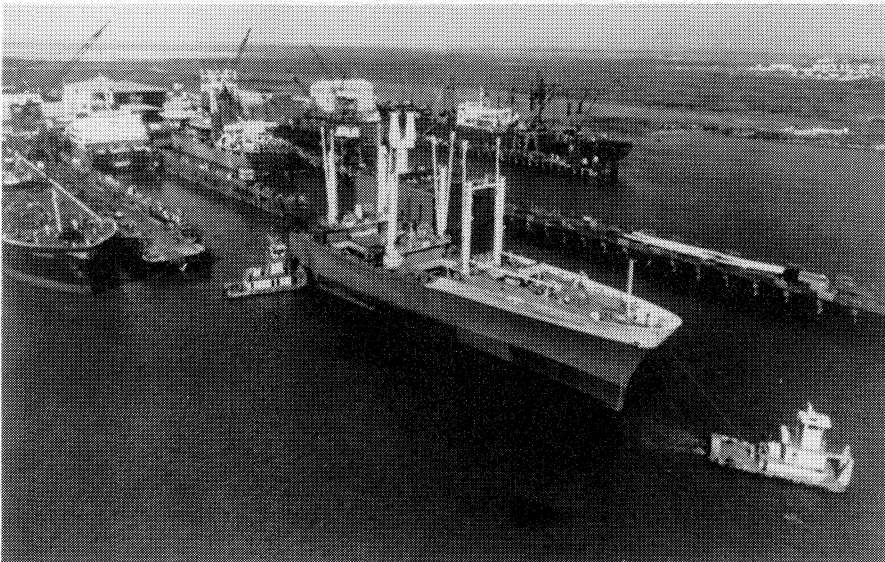
At Todd Shipyards in Galveston, Tex., tugs tow forward half of MORMACALTAIR out of dry dock so that new midbody of jumboized Moore McCormack general cargo ship can be floated in—and all sections connected.
