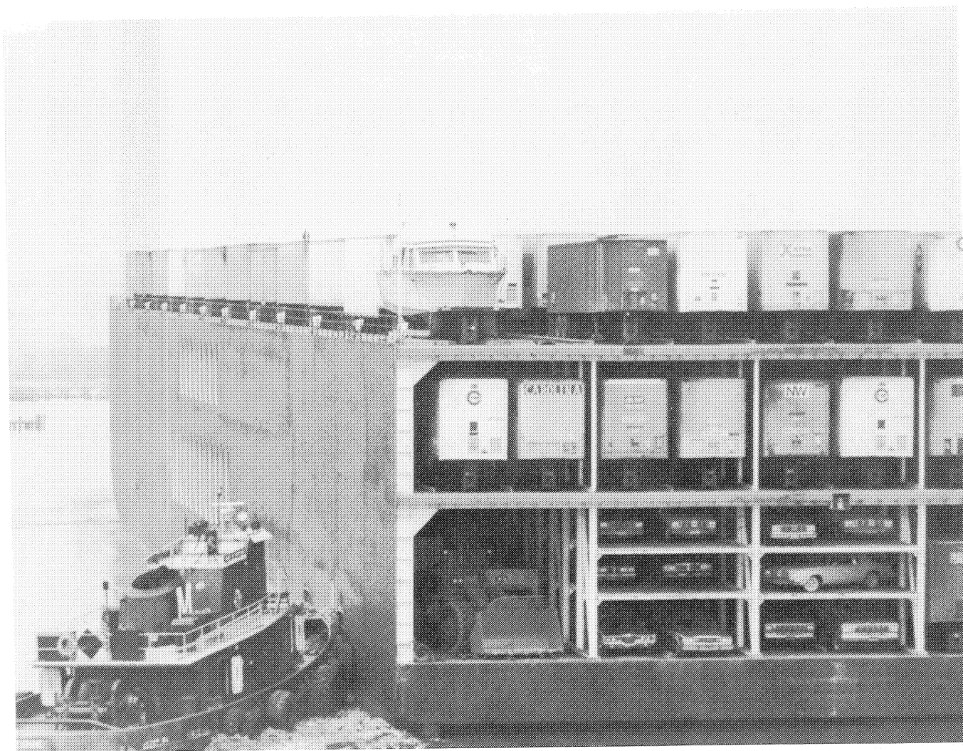
Special decks for cars add carrying capacity to Crowley Maritime/Trailer Marine Transport's EL CONQUISTADOR, one of four RO/RO barges operated between TMT home ports—Jacksonville and Miami, Fla.—and Puerto Rico. Vessels are world's largest Roll-On/Roll-Off barges.
