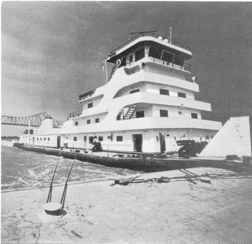
COOPERATIVE SPIRIT, at 10,500 horsepower, rated among most powerful and largest towboats operating on U.S. inland waterways, pushes tow on Mississippi River near Vicksburg, Miss. Vessel is owned and operated by Agri-Trans Corp., St. Louis, Mo.
