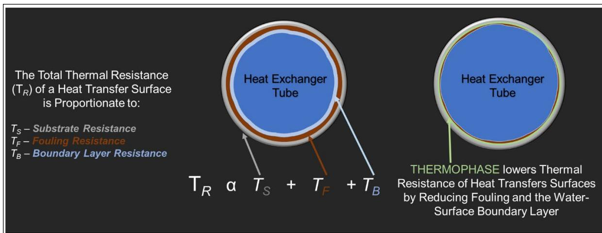
**Figure 1. THERMOPHASE Mechanism of Action.** The total thermal resistance of a heat transfer surface ( $T_R$ ) is proportional ( $\propto$ ) to the sum of the substrate resistance ( $T_S$ ), the fouling resistance ( $T_F$ ), and the boundary layer resistance ( $T_B$ ). THERMOPHASE is believed to improve heat transfer via reducing both the fouling and the boundary layer resistances.
