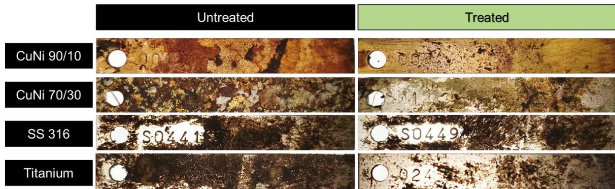
**Figure 15. Biofouling Images on Coupons.**
