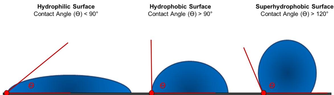
**Figure 10. Contact Angle Schematic.**
