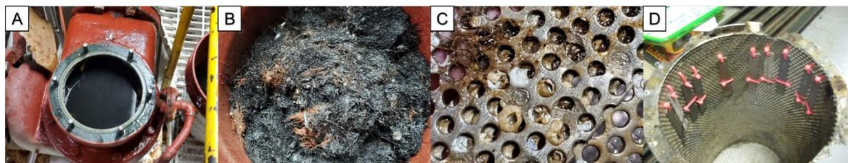
**Figure 9. Biofouling Coupon Strainer Installation.** The seawater strainer (A) was inspected prior to the summer cruise and contained an accumulation of sea waste (B). The presence of microfouling and macrofouling were apparent on the walls of the strainer (C). The coupons were suspended to the walls of the strainer (D).
