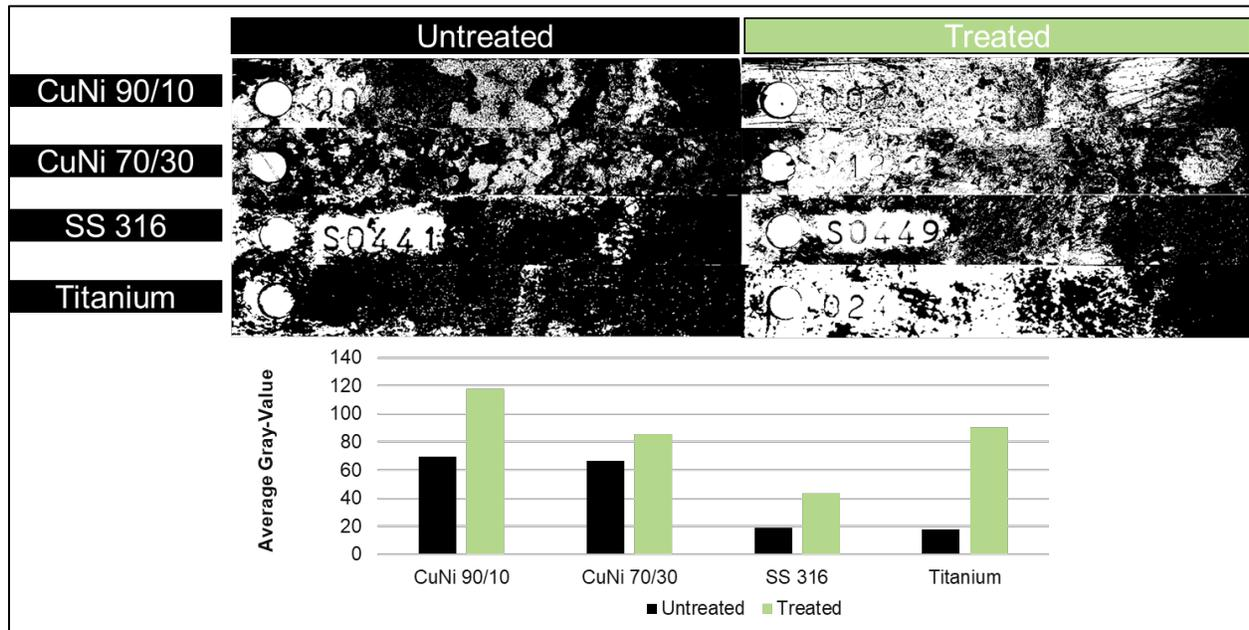
**Figure 16. Biofouling Coupon Image Analysis Summary.** The average gray value is calculated by averaging each gray value for the entire coupon area (0 is a white pixel and 255 is black pixel).
