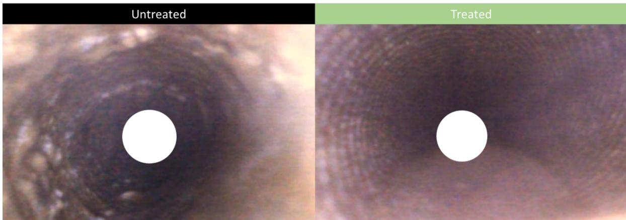
**Figure 18. Biofouling in USTS Heat Exchanger Comparison.**
