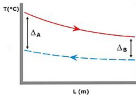
**Figure 20.** The LMTD illustrated in a countercurrent temperature profile
