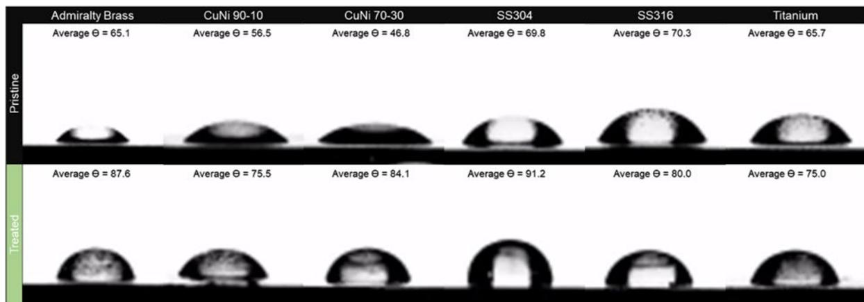
**Figure 13. Coupon Contact Angle Following THERMOPHASE Treatment.**
