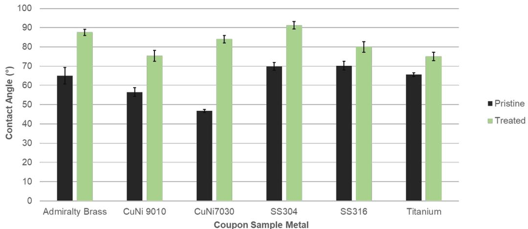
**Figure 14. Contact Angle Comparison Following THERMOPHASE Treatment.**
