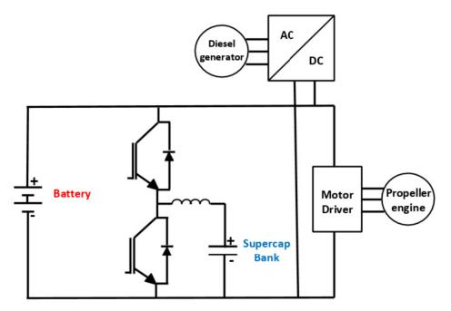
Figure 67: Supercapacitor energy storage in hybrid mechanical/electrical propulsion plant (source: Eaton)
