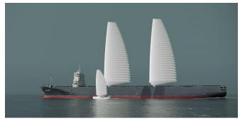
Figure 91: WISAMO inflatable sails (source: Michelin via cnn.com)
