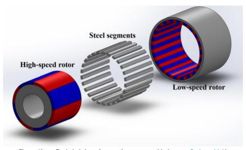
Figure 42: Exploded view of magnetic gear assembly (source: Springer Link)
