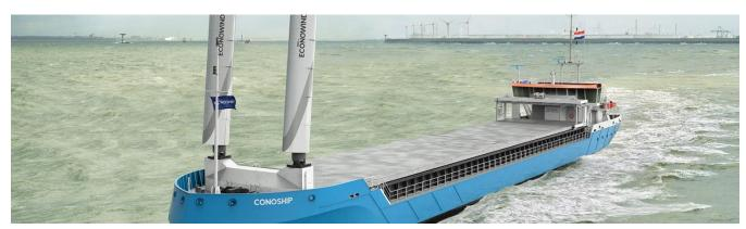
Figure 125: Conoship CIP3600 concept with diesel-electric propulsion (source: Conoship International)
