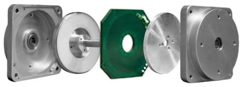
Figure 44: PCB motor stator assembly (source: Maritime Executive)
