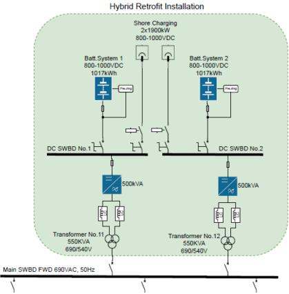
Figure 62: Battery and utility shore charging system (source: Westcon)
