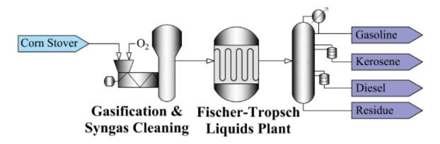
Figure 113: Fischer Tropsch synthesis using corn stover as feedstock (source: Biofuel Research Journal)
