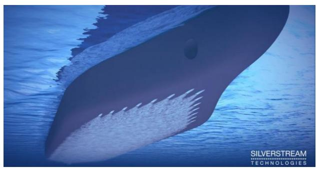
Figure 17: V-array of 14 air release units (Source: Silverstream via seatrade-maritime.com [B7])
