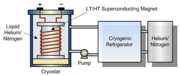
Figure 68: Superconducting magnetic energy storage illustration (source: ESES Lab)
