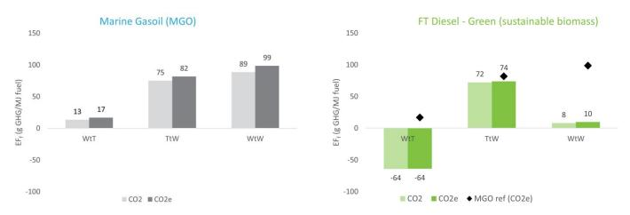
Figure 8: Comparison of WtW emissions factors for fossil-based MGO and green FTD
