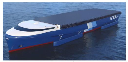
Figure 95: Ecoship 2050 concept with 9,000 m² of solar panels (source: NYK Line)
