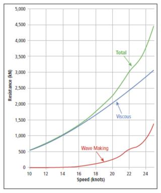
Figure 9: Typical resistance curve for a large commercial vessel (source: ABS)
