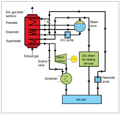
Figure 71: Process diagram for single pressure exhaust gas boiler utilizing STG (source: MAN)
