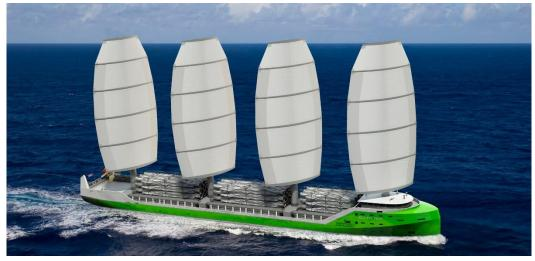
Figure 90: WASP cargo ship concept (source: Dykstra)
