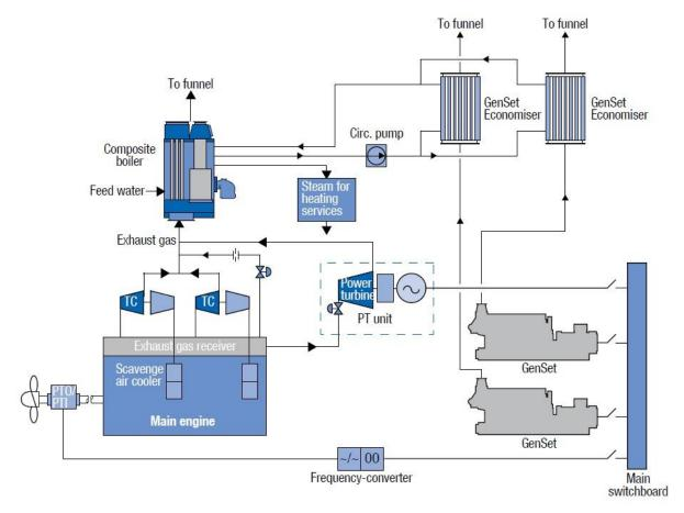
Figure 69: Power turbine generator schematic (source: MAN)
