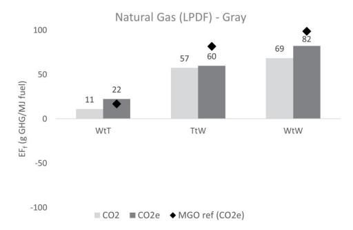
Figure 3: Lifecycle CO<sub>2</sub> and CO<sub>2</sub>e emission factors for fossil-based natural gas, diesel cycle (low pressure dual fuel – LPDF)
