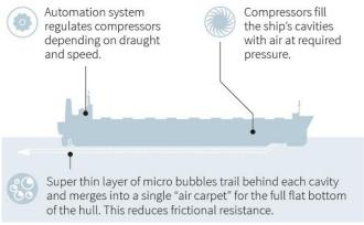
Figure 16: Simplified representation of air lubrication process (Source: vesselfinder.net)
