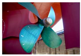
Figure 19: MAITA propeller (Source: Oshima [B9])
