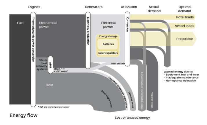
Figure 1: Energy breakdown for a diesel-electric vessel (source: ABB)
