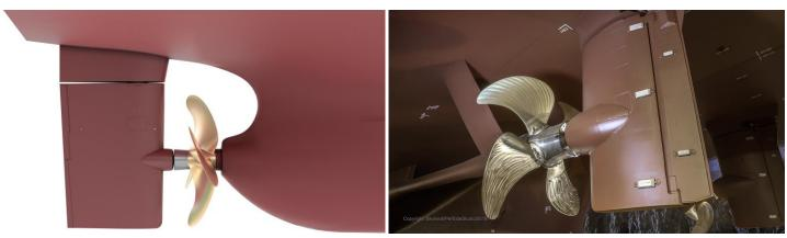
Figure 34: Kongsberg Promas propulsion system with costa bulb (left, source: Kongsberg [B18]) and Brunvoll integrated costa bulb (right, source: Brunvoll [B19])
