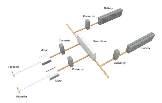
Figure 51: Typical battery (all-electric) topology with AC switchboard (source: MAN-ES)
