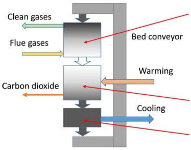
The separation takes place at a temperature of about -100°C.
