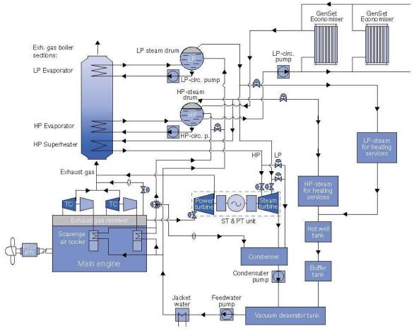
Figure 73: Combined PTG + STG schematic (source: MAN)
