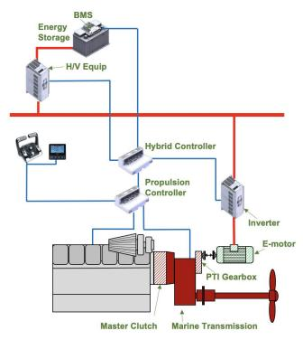
Figure 50: Parallel hybrid electric plant (source: TwinDisc [B31])
