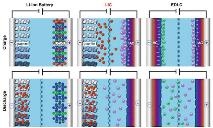
Figure 66: EDLC and LIC supercapacitor processes compared to li-ion batteries (source: Naoi)
