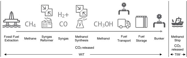
Figure 114: Methanol CO<sub>2</sub> lifecycle from natural gas and steam methane reformation (gray)
