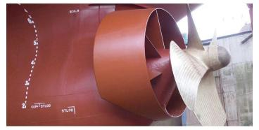
Figure 29: Becker Mewis Duct (source: Becker Marine Systems [B12])
