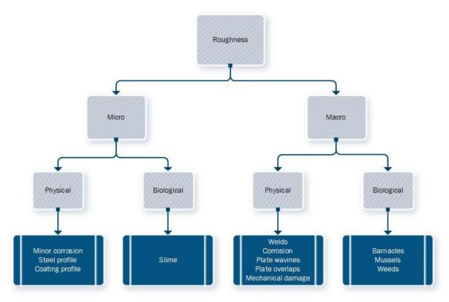
Figure 10: Types of surface roughness affecting hull friction
