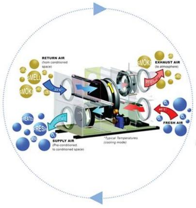
Figure 79: Energy recovery ventilator using enthalpy wheel (source: DRI)
