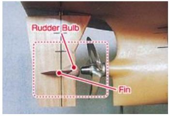
Figure 31: Rudder thrust fins paired with rudder bulb (source: Kawasaki)
