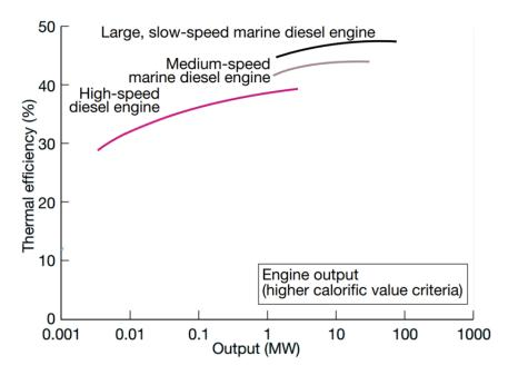
Figure 53: Thermal efficiencies of various size marine diesel engines from 2010 (source: adapted from MHI Technical Review).
