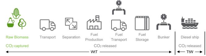
Figure 4: Typical emissions lifecycle of bio-fuel type diesel for marine use
