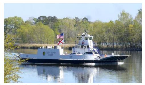
Figure 56: Gee's Bend Ferry, the first all-electric ferry to operate in the US (source: workboat.com)
