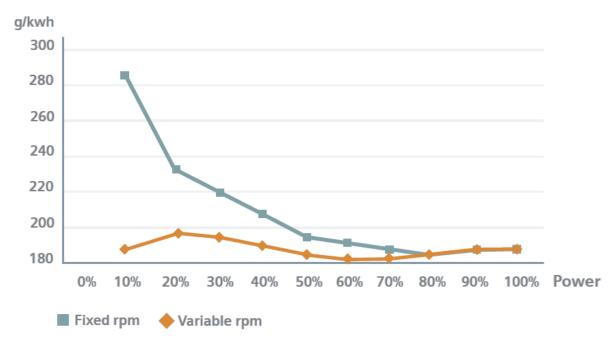
Figure 39: Specific fuel consumption for variable speed vs fixed speed diesel-generators (source: Siemens)
