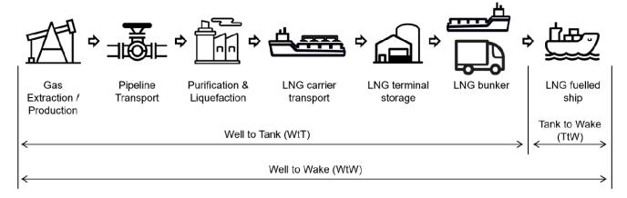
Figure 2: Typical emissions lifecycle of fossil-based LNG for marine use (Source: Journal of Marine Science and Engineering)
