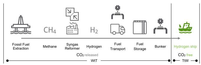
Figure 104: Hydrogen CO<sub>2</sub> lifecycle from natural gas and steam methane reformation (gray)
