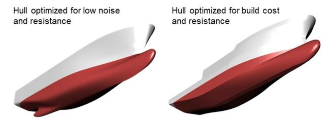
Figure 15: Comparison of two research vessel hull forms optimized to minimize resistance: low noise on left versus build cost on right (Source: Glosten)
