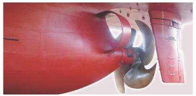
Figure 28: A Schneekluth wake equalizing duct, a type of pre-swirl duct (source: Wartsila [B15])
