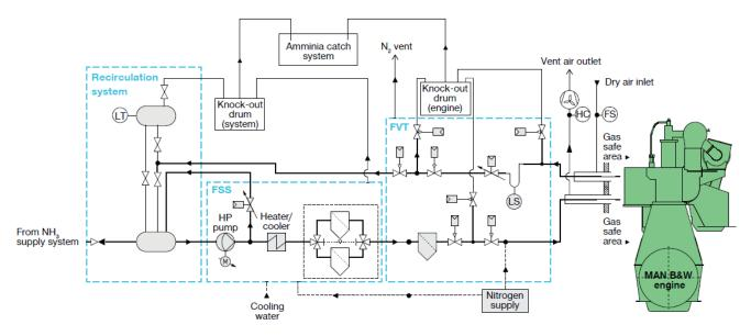
Figure 118: Concept diagram of ammonia high-pressure fuel supply system for 2-stroke, dual fuel engine (source: MAN-ES)
