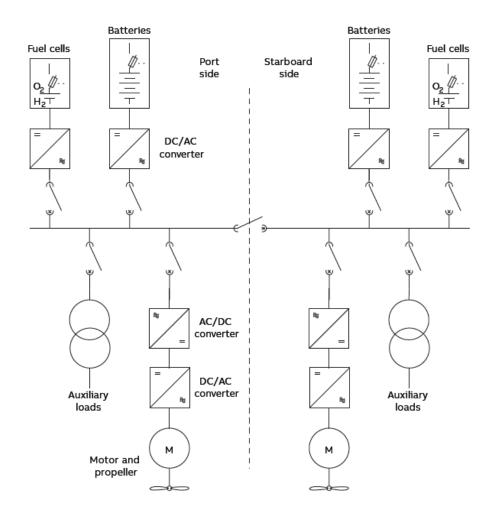
Figure 144: Conceptual one-line diagram with battery-electric power using hydrogen fuel cells (source: ABB)
