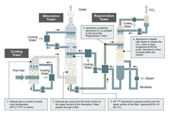
Figure 126: Absorption carbon capture process (source: MHI)
