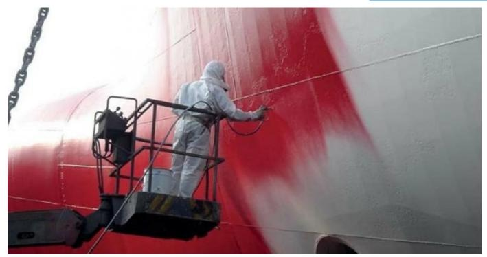
Figure 11: Coating being applied to the vessel hull (Source: Seatrade Maritime News)
