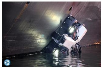
Figure 13: A Fleet Cleaner robot cleans the side of a vessel's hull (Source: Fleet Cleaner [B5])
