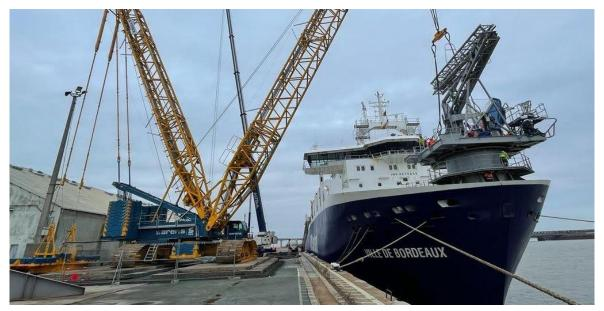
Figure 82: Seawing's kite sail installation on Ville de Bordeaux, IMO no. 9270842 (source: heavyliftnews.com)
