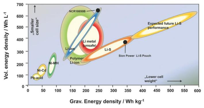
Figure 55: Energy density comparison of various battery chemistries (source: Hagen, et al.)
