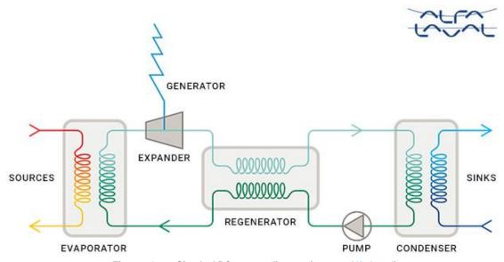
Figure 74: Simple ORC system diagram (source: Alfa Laval)
