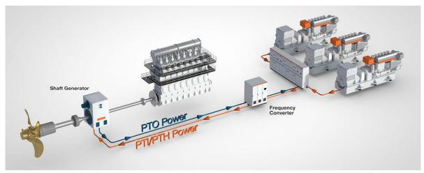
Figure 41: Shaft-generator shown in both PTO and PTI operation (source: Wartsila [B25])
