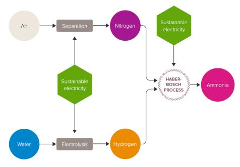
Figure 110: Green ammonia pathway from water electrolysis of hydrogen and air separation of nitrogen using renewable electricity (source: The Royal Society)
