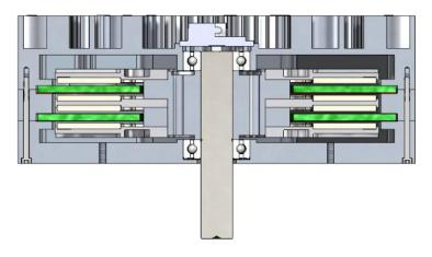
Figure 46: Stacked PCB stators within one motor housing (source: ECM)
