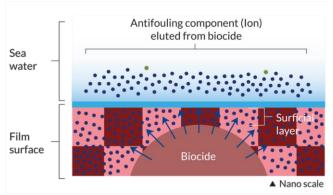
Figure 12: Nanocoating representation (source: Nippon Paint Marine)
