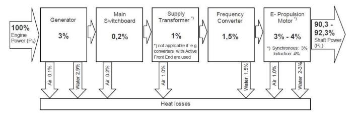
Figure 38: Typical energy losses of a diesel-electric power generation and propulsion plant (source: MAN)
