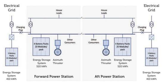
Figure 59: Line diagram of the Ampere drive systems (image courtesy of Corvus Energy)
