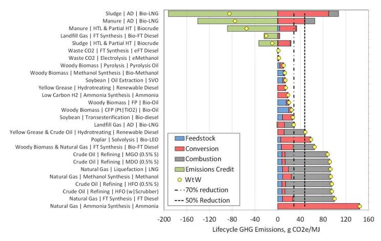
Figure 112: Biofuels and their WtW CO<sub>2</sub>e emissions (source: Argonne GREET data)
