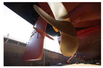
Figure 30: Hyundai (HHI) thrust fins attached to a ship's rudder (source: HHI)
