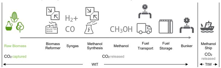
Figure 115: Methanol CO<sub>2</sub> lifecycle from direct biomass gasification/reformation (green)
