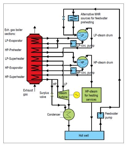
Figure 72: Process diagram for dual pressure exhaust gas boiler utilizing STG (source: MAN)
