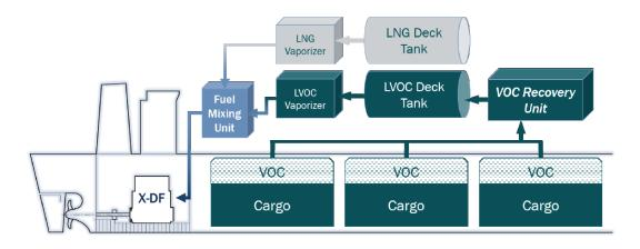
Figure 102: Concept diagram of WinGD VOC recovery fuel system (source: WinGD)
