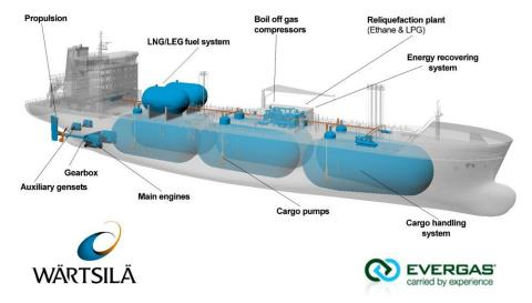
Figure 101: Evergas product carrier converted to burn ethane, stored in liquid form (source: Wartsila)
