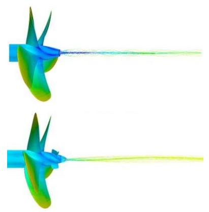
Figure 36: Comparison of propeller streamlines: without PBCF on top, with PBCF on bottom (source: Applied Ocean Research)
