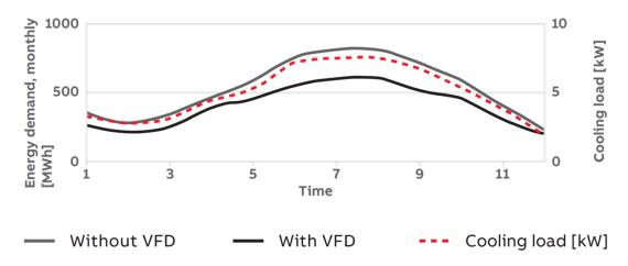
Figure 78: Energy savings with VFD-controlled chiller compressors (source: ABB)
