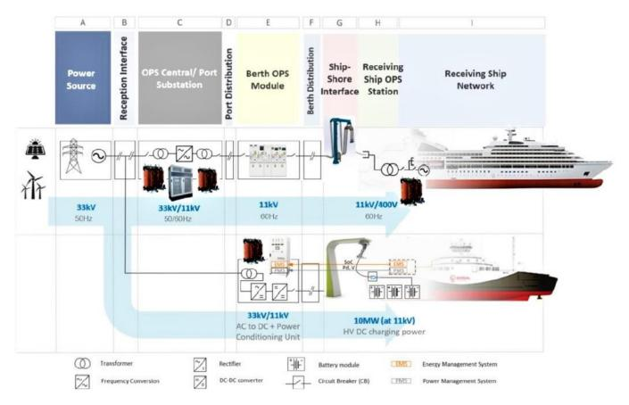
Figure 63: Generic perspective of key infrastructure elements for shore power (source: EMSA)
