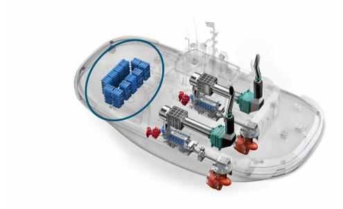
Figure 143: Hydrotug with compressed hydrogen shown below aft working deck (source: rivieramm.com)
