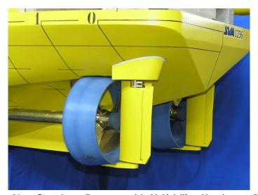
Figure 21: Ducted propellers on a model with high-lift rudders (source: SVA)
