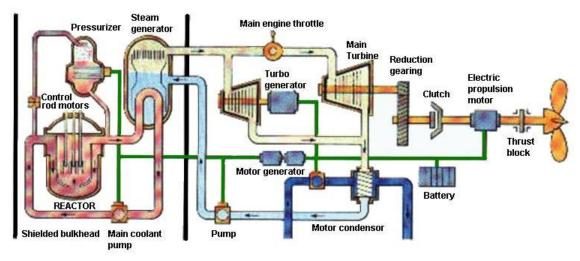
Figure 133: Typical Shipboard PWR Propulsion Plant (source: fas.org)
