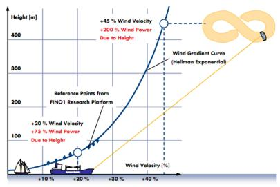
Figure 81: Kite sail flow characteristics (source: Skysails via wattnow.org)
