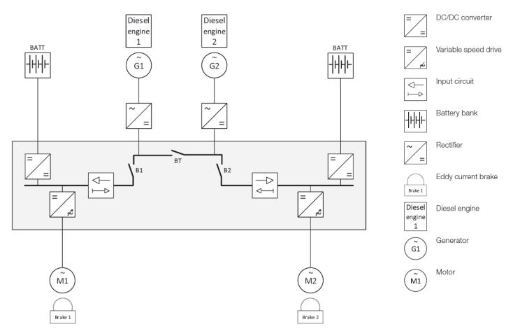
Figure 142: Simple hybrid mechanical/electric single line diagram, minus shore power charging electronics (Source: adapted from ABB)
