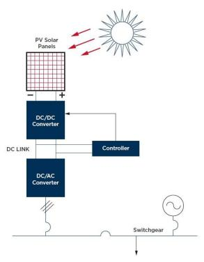
Figure 96: Conceptual one-line diagram for PV solar panel integration (source: ABS)
