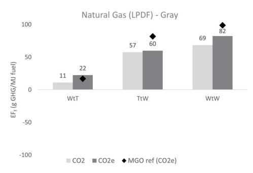
Figure 98: Lifecycle CO₂ and CO₂e emission factors for fossil-based natural gas, diesel cycle (low pressure dual fuel, LPDF)
