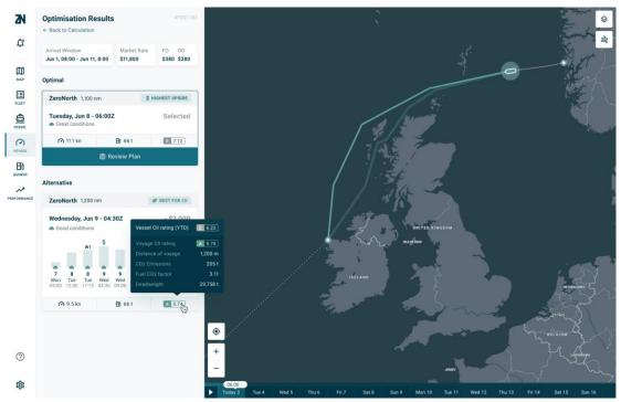
Figure 140: Screenshot example from a commercial weather routing system. (source: marineinsight.com)
