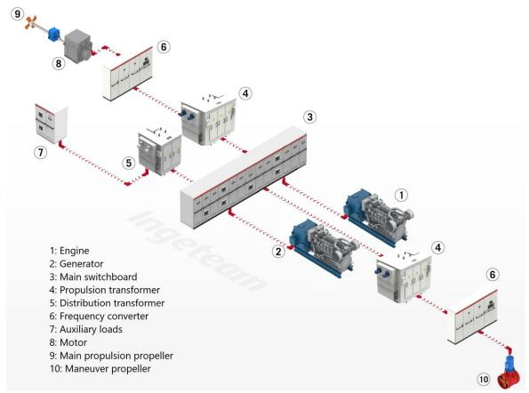
Figure 37: Typical diesel-electric propulsion topology with AC switchboard (source: Ingeteam [B22])
