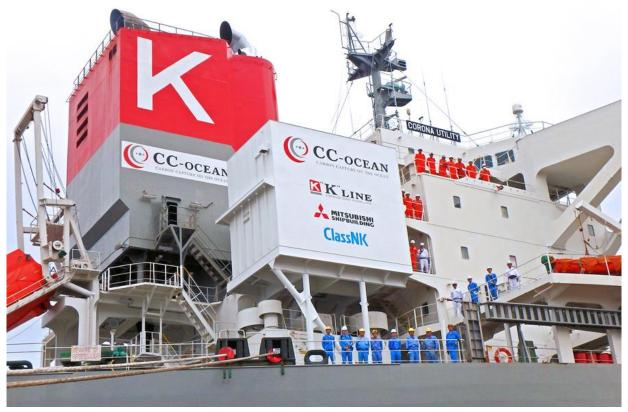
Figure 130: MHI absorption carbon capture system installed as part of CC-Ocean project (source: MHI)
