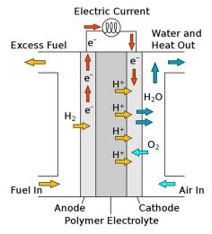
Figure 121: Basic fuel cell chemistry diagram (source: energyeducation.ca)
