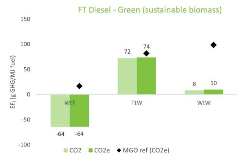
Figure 5: Lifecycle CO<sub>2</sub> and CO<sub>2</sub>e emission factors for green (sustainable biomass) FTD
