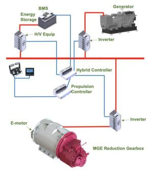
Figure 49: Series hybrid electric plant (source: TwinDisc [B31])
