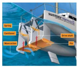
Figure 92: Suntory Mermaid hydrofoil propulsion technology (source: proboat.com)
