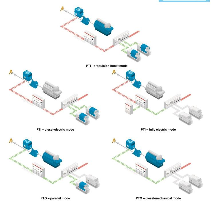
Figure 40: Various PTI and PTO topologies (source: Ingeteam [B22])
