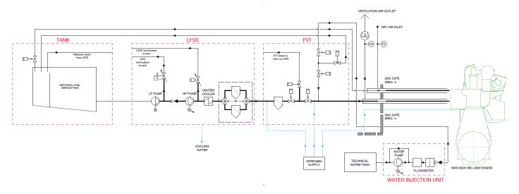
Figure 120: Concept diagram of methanol high-pressure fuel supply system, 2-stroke dual fuel (source: MAN-ES)
