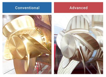
Figure 35: Conventional [left] and advanced [right] PBCF (source: PBCF [B20])
