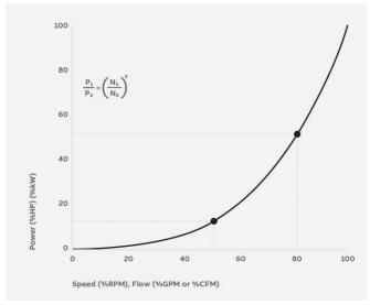
Figure 77: Speed vs flow relationship to power (source: ABB)
