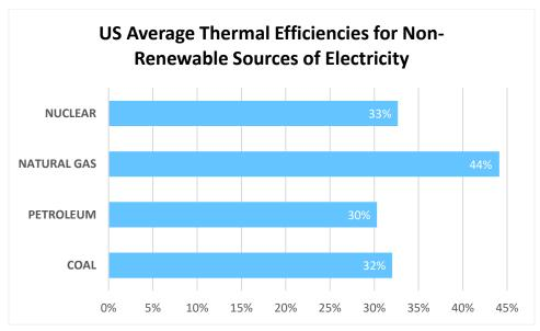
Figure 52: Thermal efficiencies for US non-renewable grid power, 2020 (source: Energy Information Administration (EIA))
