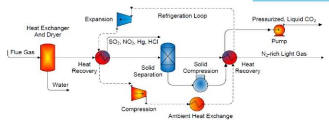
Figure 127: Cryogenic carbon capture process (source: NETL)
