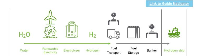
Figure 105: Hydrogen CO<sub>2</sub> lifecycle from renewable water electrolysis (green)
