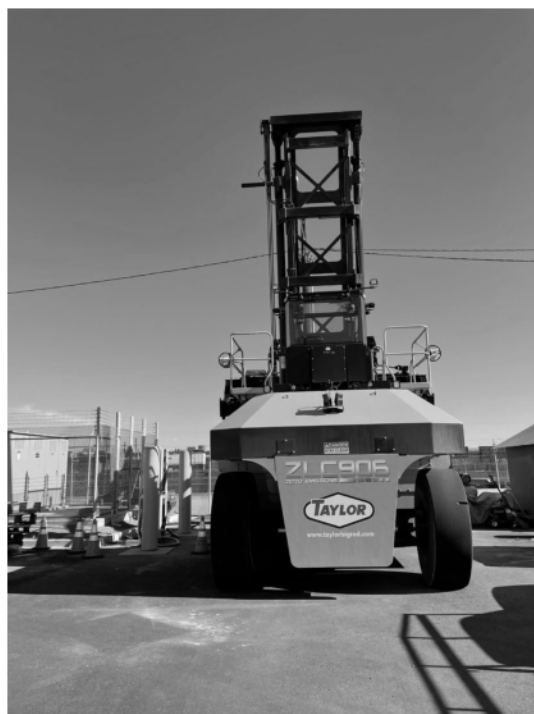
Battery-Electric Yard Equipment (Top Pick Stacker) at the Port of Oakland
