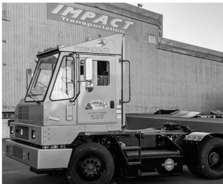
Battery-Electric Yard Equipment (Hostler) at Port of Oakland
