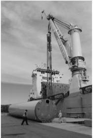
Figure 1: Wind tower loading
