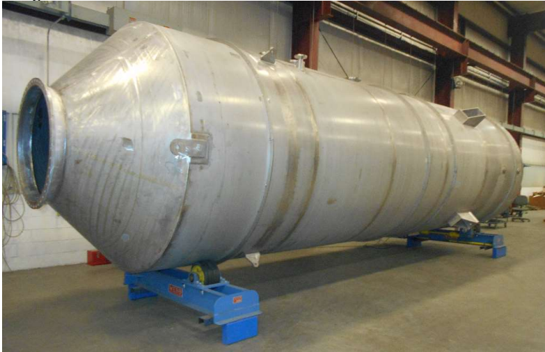
Scrubber vessel during fabrication
