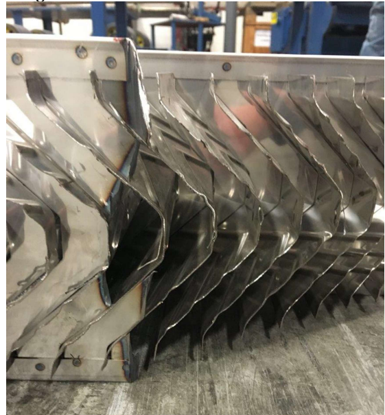
Chevron style droplet separators
