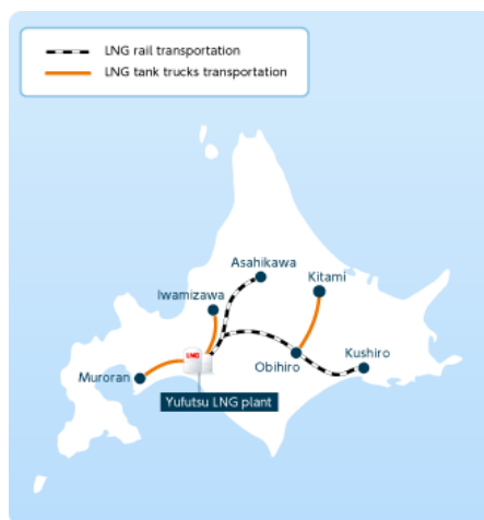
Figure 11: Natural gas marine-rail-truck supply chain Hokkaido Island, Japan. (Japan Petroleum Exploration Co., Ltd., 2014)
